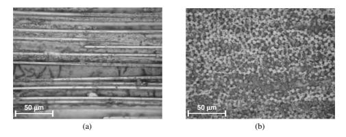
**Figure 9.** Optical micrographs after sequential exposure to 500 h of UV radiation followed by 500 h of condensation: (a) edge of a  $[0]_8$  specimen; (b) edge of a  $[90]_8$  specimen.
