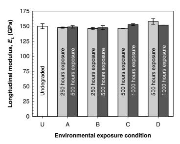
**Figure 15.** Variation of longitudinal modulus,  $E_L$ , for exposure to UV radiation and/or condensation: U – undegraded with no exposure, A – exposure to only UV radiation, B – exposure to only condensation, C – sequential exposure, and D – cyclic exposure.
