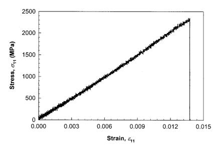
Figure 13. A typical stress-strain plot for uniaxial tension testing of a [0/90]<sub>2S</sub> specimen.
