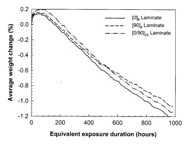
Figure 5. Change in specimen weight, as a function of time, for cyclic exposure to both UV radiation and condensation.
