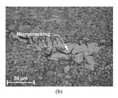
**Figure 7.** Optical micrographs after 500 h of exposure to UV radiation: (a) edge of a  $[0]_8$  specimen at high magnification; (b) edge of a  $[90]_8$  specimen at high magnification.
