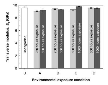
**Figure 16.** Variation of transverse modulus,  $E_T$ , for exposure to UV radiation and/or condensation: U – undegraded with no exposure, A – exposure to only UV radiation, B – exposure to only condensation, C – sequential exposure, and D – cyclic exposure.
