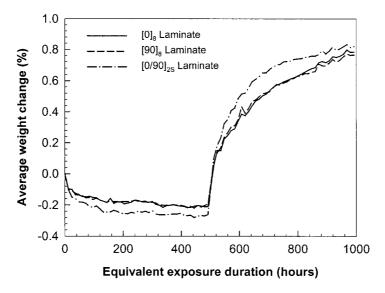
Figure 4. Change in specimen weight, as a function of time, for sequential exposure to UV radiation followed by condensation.
