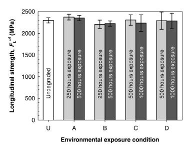
**Figure 18.** Variation of longitudinal tensile strength,  $F_{L}^{ut}$ , for exposure to UV radiation and/or condensation: U – undegraded with no exposure, A – exposure to only UV radiation, B – exposure to only condensation, C – sequential exposure, and D – cyclic exposure.
