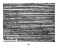
**Figure 6.** Optical micrographs for composite specimen prior to environmental exposure: (a) surface of  $[0]_8$  specimen; (b) edge of a  $[0]_8$  specimen at high magnification.
