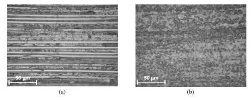
**Figure 8.** Optical micrographs after 500 h of exposure to condensation: (a) edge of a  $[0]_8$  specimen at high magnification; (b) edge of a  $[90]_8$  specimen at high magnification.
