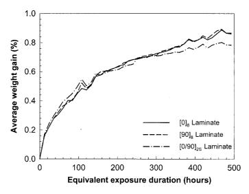
Figure 3. Change in specimen weight, as a function of time, for exposure to only condensation.
