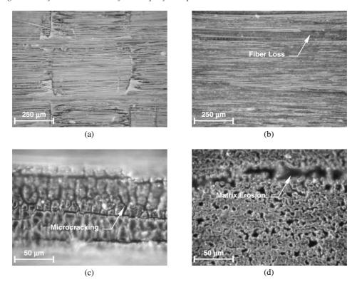
**Figure 10.** Optical micrographs after  $1000 \, h$  of cyclic exposure to both UV radiation and condensation: (a) surface of a  $[0]_8$  specimen; (b) edge of a  $[0]_8$  specimen; (c) edge of a  $[0]_8$  specimen at higher magnification; (d) edge of a  $[90]_8$  specimen at higher magnification.
