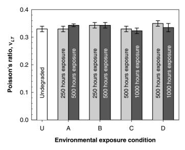
**Figure 17.** Variation of major Poisson's ratio,  $v_{LT}$ , for exposure to UV radiation and/or condensation: U – undegraded with no exposure, A – exposure to only UV radiation, B – exposure to only condensation, C – sequential exposure, and D – cyclic exposure.
