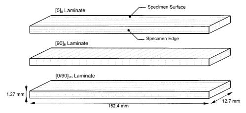
Figure 1. Schematic representation of the three different specimen configurations employed for investigation of degradation by UV radiation and/or condensation.
