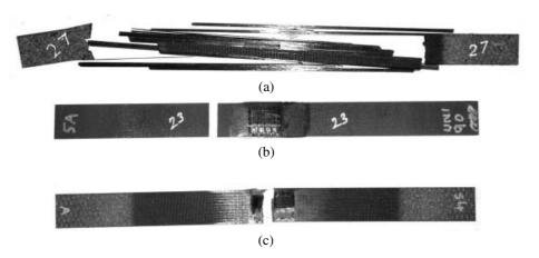
**Figure 14.** Failure modes under uniaxial tension: (a) axial splitting for  $[0]_8$  specimens, (b) transverse matrix failure for  $[90]_8$  specimens; (c) fiber breakage for  $[0/90]_{2S}$  specimens.
