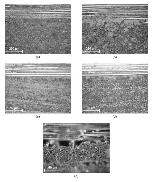
**Figure 11.** Optical micrographs for the edge of [0/90]<sub>2S</sub> specimens exposed to various environments: (a) undegraded; (b) exposed to only UV radiation; (c) exposed to only condensation; (d) sequentially exposed to UV radiation followed by condensation; (e) cyclically exposed to UV radiation and condensation.
