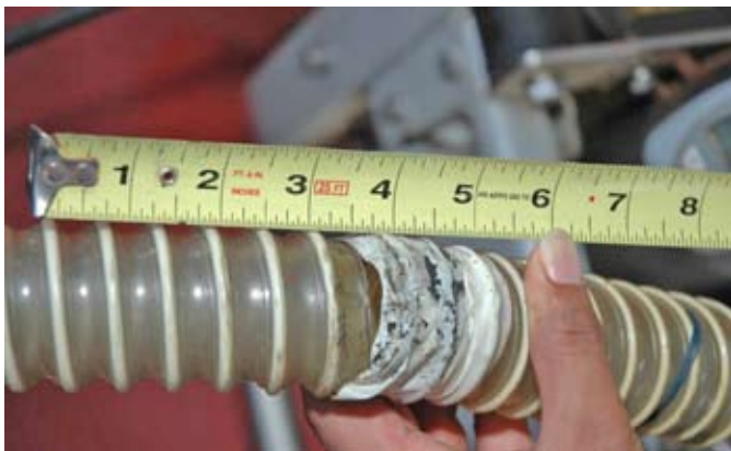
Defective intake hose with tape patches on the boat
