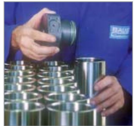
Final separator assembly at BAUER
