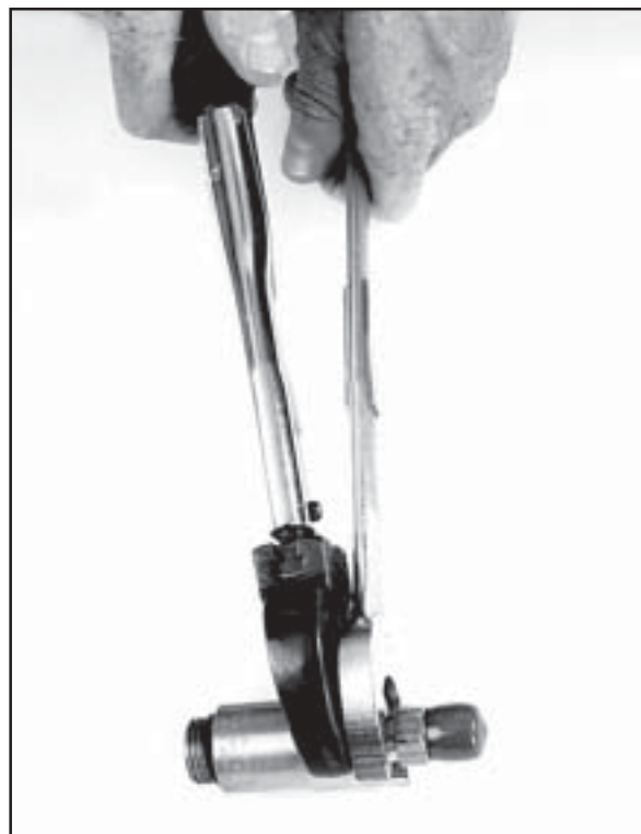
Fig. 5.10 If no vise is available you may use two wrenches to disassemble the valve.
