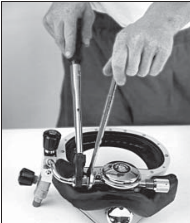
Fig. 6.23 Loosen the jam nut prior to removing the bent tube.
