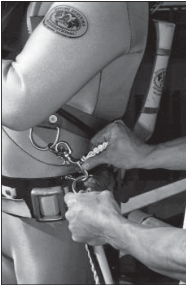
Fig. 2.18 The umbilical must always be attached to the diver's harness with some type of clip to prevent a direct pull on the diver's mask.
