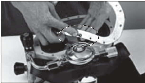
Fig. 6.8 Be sure to install the small O-ring that seals the nose block device on the back side of the port retainer.
