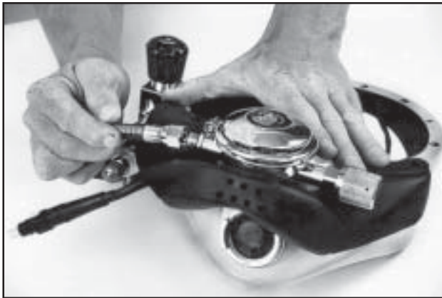
Fig. 6.21 The hose assembly must be removed prior to removal of the side block.
