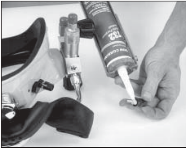
Fig. 6.20 Apply fresh RTV silicone sealant to the communications posts prior to installation.
