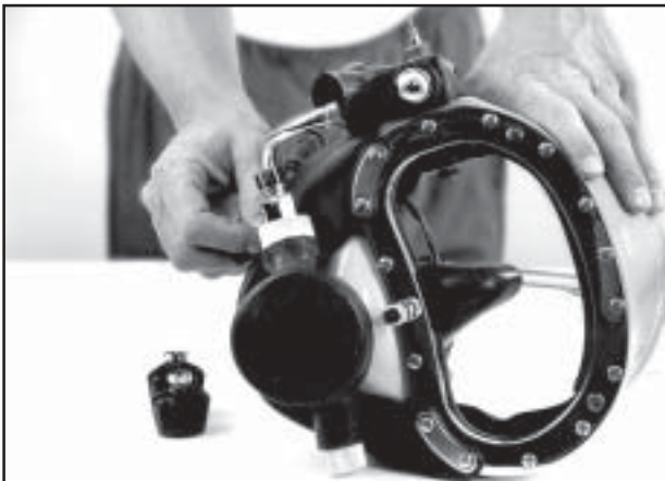
Fig. 7.4 Install the PVC flanges.
