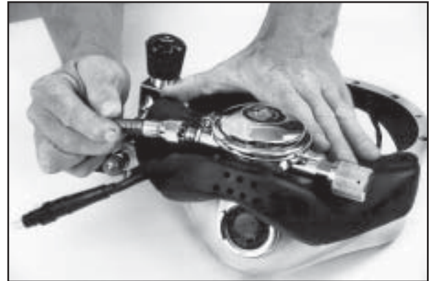
Fig. 6.42 Replacing an "A" regulator hose.
