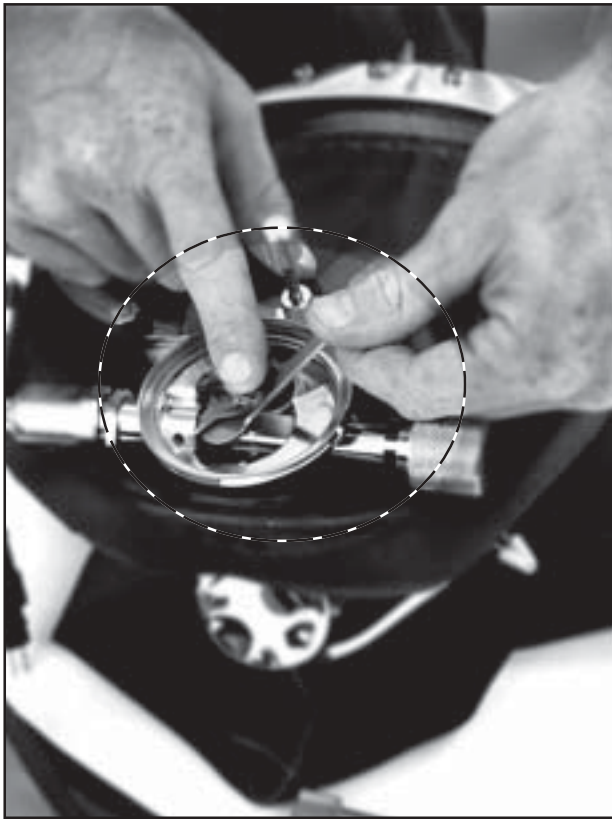
Fig. 5.27 Use the round end of the adjustment wrench for leverage in bending the lever down.
