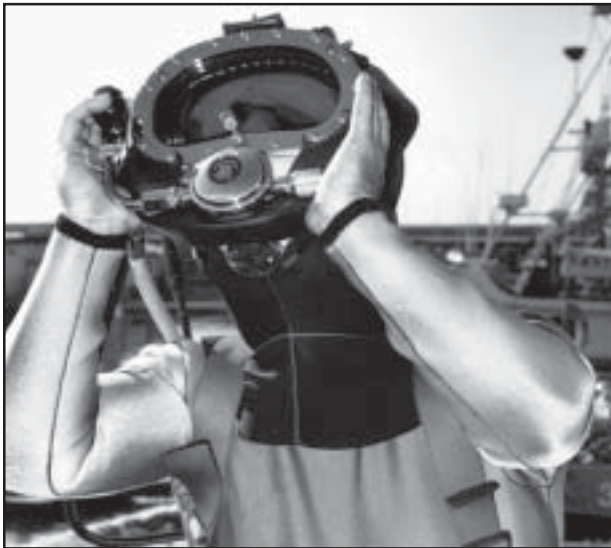
Fig. 2.20 The diver should be capable of removing the Band Mask by himself.
