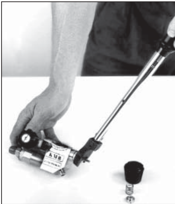
Fig. 6.35 Removal of the valve bonnet.
