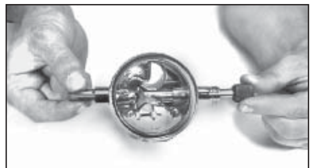
Fig. 6.63 Use the KMDSI socket wrench to turn the nut on the inlet valve.
