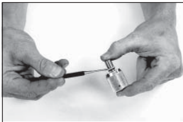
Fig. 5.20 Replace the washer and O-ring if necessary.
