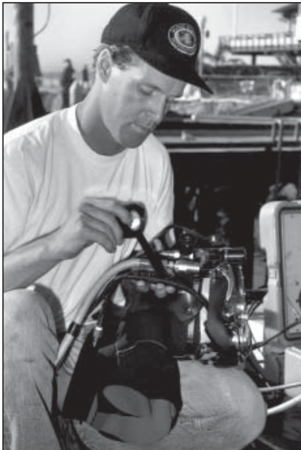
Fig. 2.5 Tape the two mating waterproof connectors together with electrical tape prior to diving.
