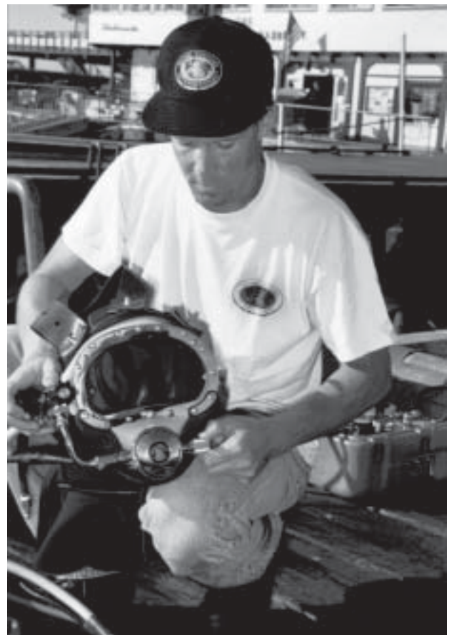
Fig.2.2 Moving parts, such as the regulator adjustment knob must be checked before the Band Mask is put on line.
