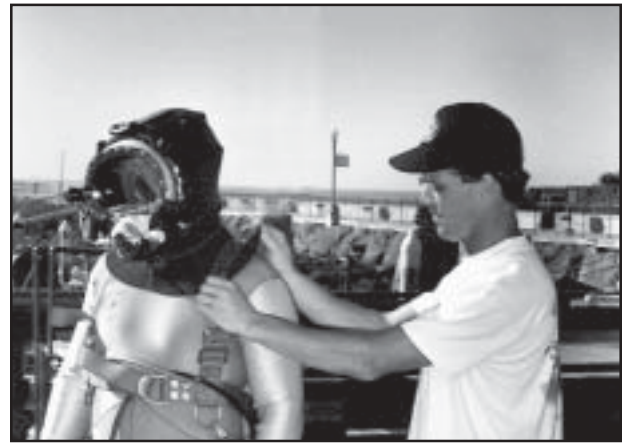
Fig. 2.17 To keep the bib of the hood from the mask from floating up, it may be tucked underneath the straps of your diving harness.
