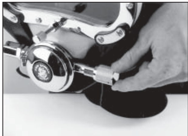
Fig. 5.13 Back the regulator adjustment knob all the way out when the mask will not be used for more than a few hours.
