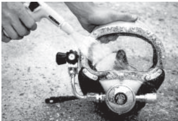
Fig. 5.5 The mask should be rinsed thoroughly with fresh water at the end of each diving day.
