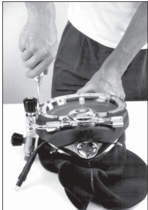
Fig. 6.9 The port retainer screws must be accurately tightened with a torque screwdriver.
