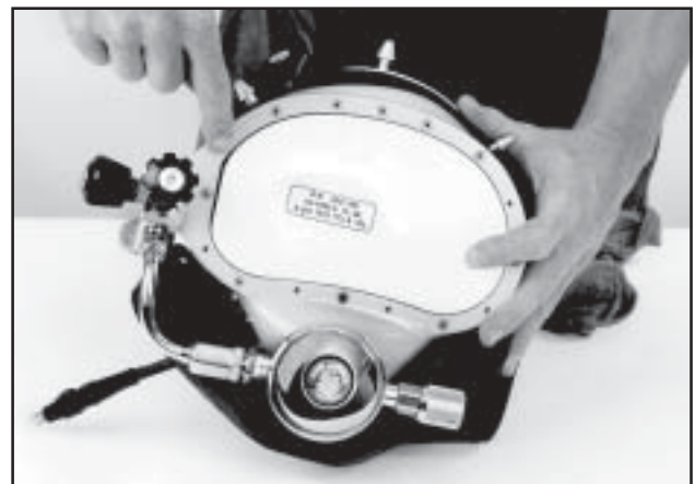
Fig. 6.1 The face port from the KMB 28 will not fit properly in a KMB 18A/B. NOTE THE GAP WHERE THE PORT DOES NOT PROPERLY FILL THE SPACE.
