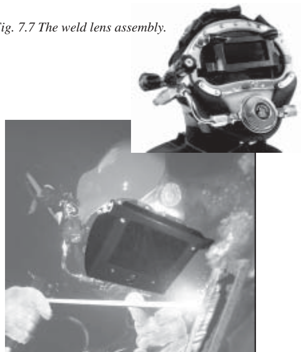
Fig. 7.8 The weld shield assembly.
