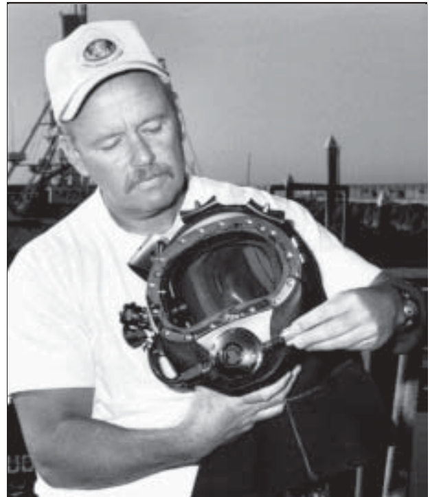
Fig. 2.6 Screw in the regulator adjustment knob prior to turning on the diver's breathing gas.
