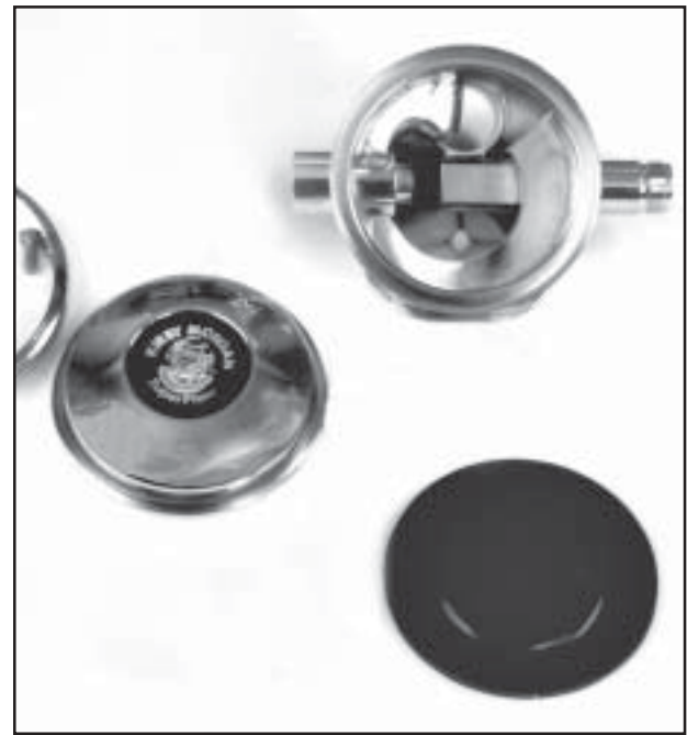
Fig. 5.15 Inspect the diaphragm.
