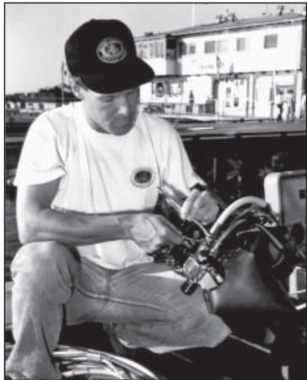
Fig. 2.4 Always use two wrenches to connect the umbilical to the KMB 18A/B or 28.
