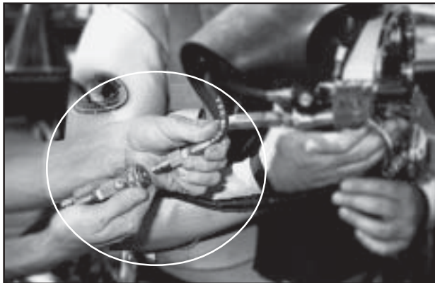
Fig. 7.8 A quick disconnect will make it simpler to hook up your bail-out to your mask.
