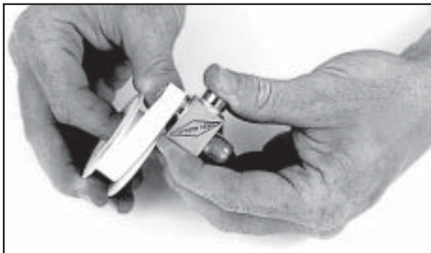
Fig. 6.38 The tapered pipe thread end of the auxiliary valve must be wrapped properly with Teflon tape prior to installation.
