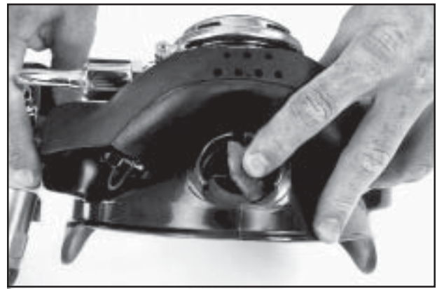
Fig. 6.56 Note how the main exhaust body is molded into the frame on the KMB 28.
