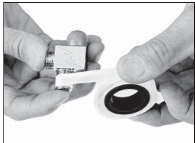
Fig. 6.27 Wrap the pipe threads with pipe tape prior to reinstalling the valve body.
