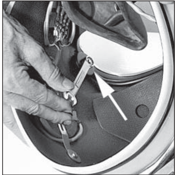
Fig. 6.7 Remove the nut that secures the air train.
