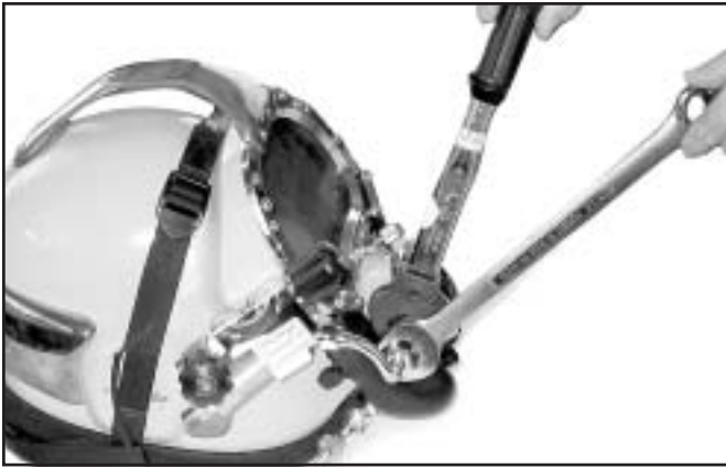
Fig. 6.51 Always use a torque wrench and a 7/8" open end wrench to Properly torque the jam nut (131b)
