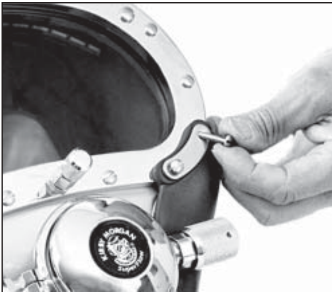
Fig. 7.16 the kidney plate screws, like any screws that go through the port retainer, must be tightened with a torque screwdriver.
