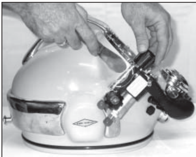
Fig. 6.9 Use a putty knife to separate the block from the helmet shell.
