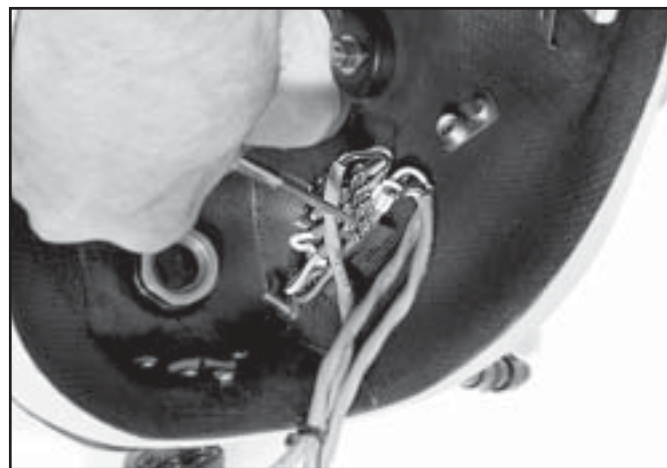
Fig. 7.20 The terminal block is where the earphones and microphone will be connected inside the helmet.
