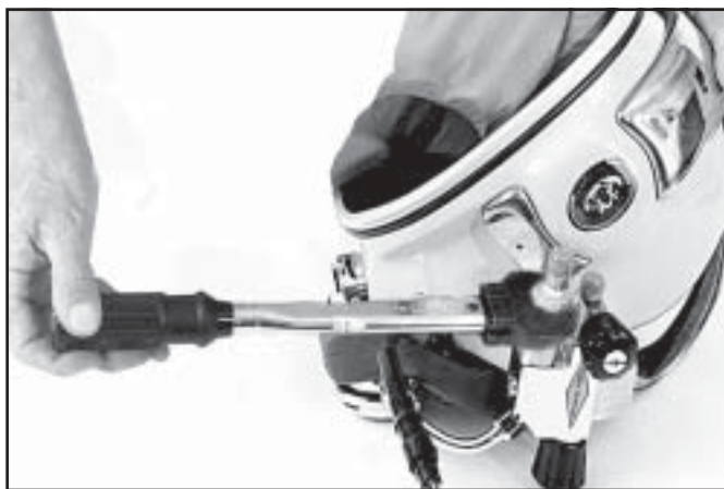
Fig. 6.4 Tighten the one way valve to 24inch lbs (270kg.cm) with torque wrench
