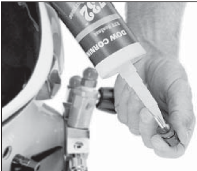
Fig. 7.24 Apply fresh RTV to the communications posts.
