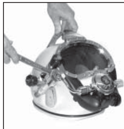
Fig. 6.5 On the SuperLite-17b, you must disconnect the bent tube to remove the side block.
