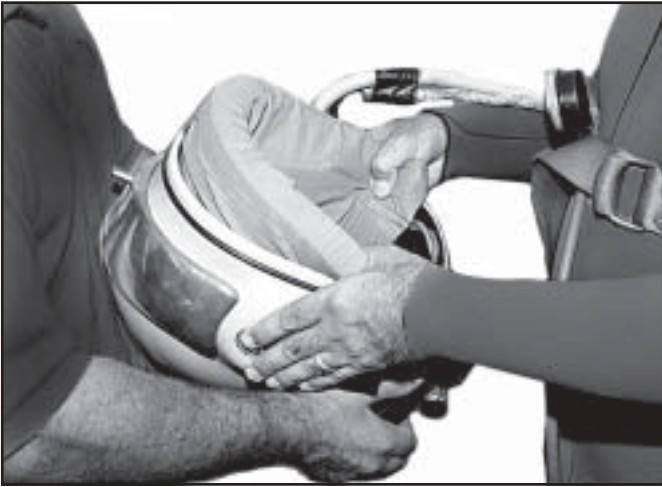
Fig. 2.14 Grab the head cushion and spread it while grasping the side of the helmet and holding the chin strap.
