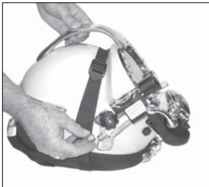
Fig. 5.2 Cover the air inlet and auxiliary valve openings with dust caps when not in use.
