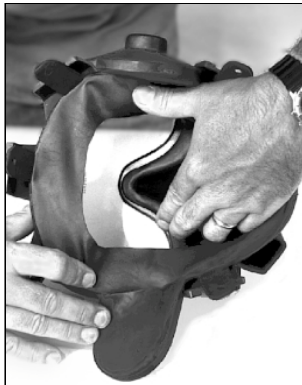
Check the seating of the mask seal and lens clamps on the inside of the mask.
