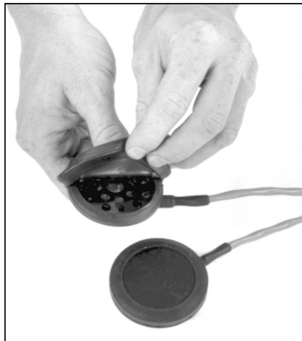
Remove the outer earphone covers and allow all the parts to dry.
