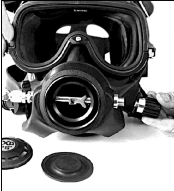
The adjustment assembly is removed after the packing nut is loosened.
