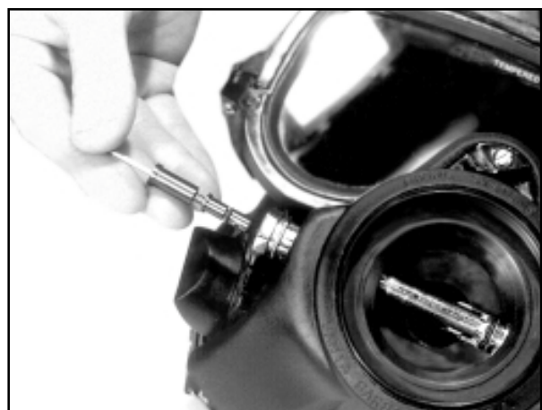
Install the inlet valve.
