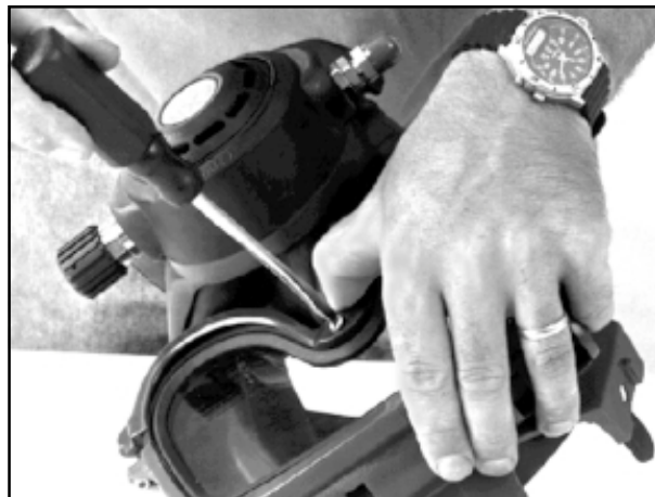
Remove the screw at the nosepiece.
