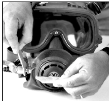
Use the spanner wrench to depress the purge button while turning the nipple to adjust the regulator
