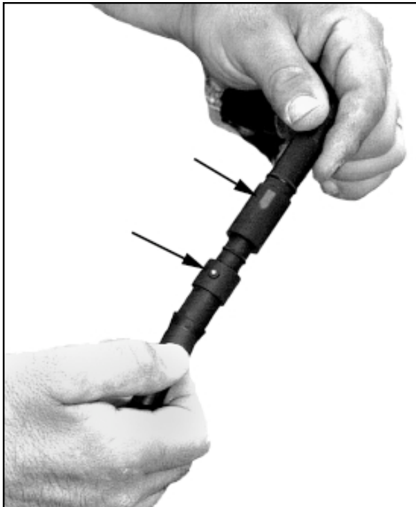
Align the key on the male connector with the yellow mark on the female connector.
