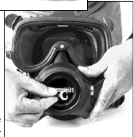
Remove the roller lever arm.
