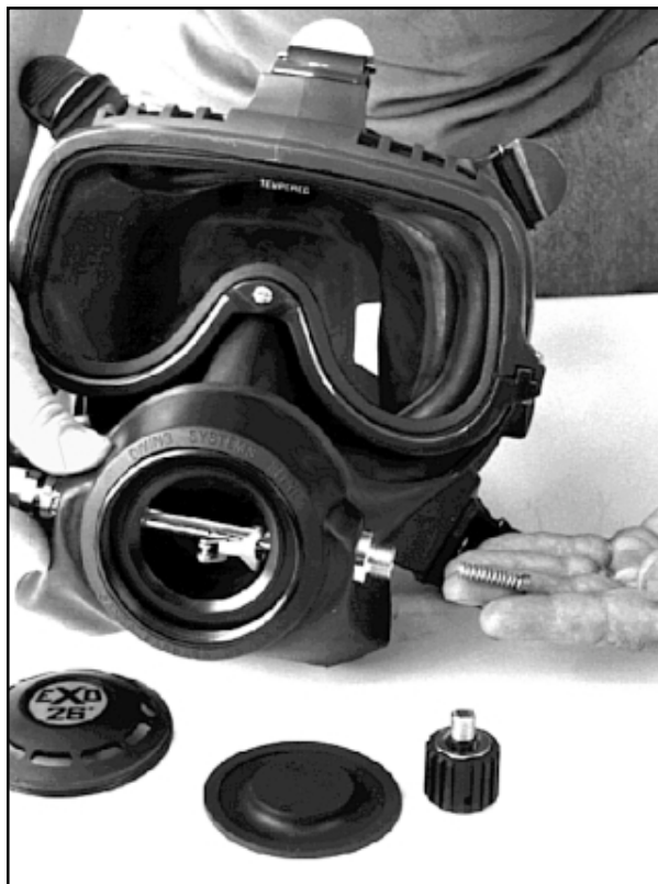
Remove the spring and spacer.
