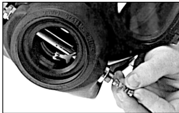
Install the spacers and spring.
