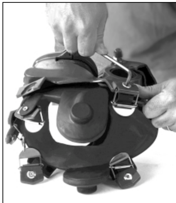
Use a \frac{3}{16} " Allen wrench to tighten the “T” nuts.
