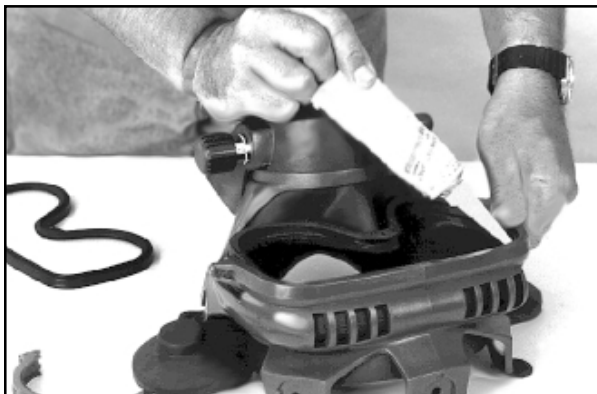
Apply silicone grease to the mask seal.
