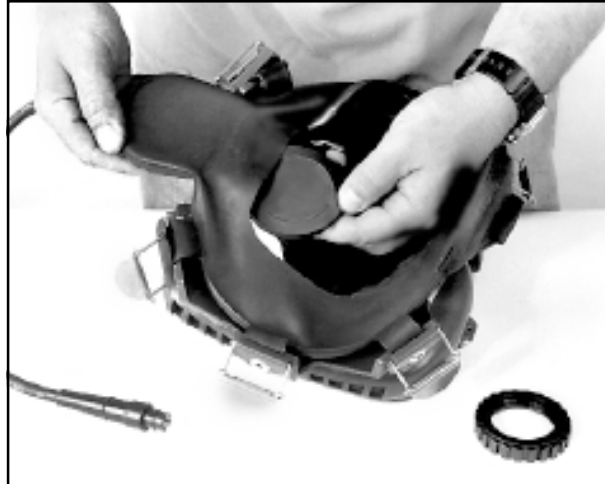
Remove the earphone assembly.
