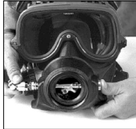
Push the main tube out enough to allow the lever arm to be removed.
