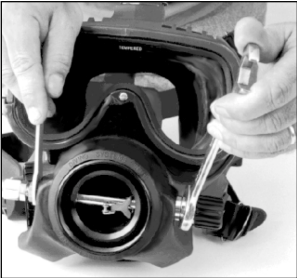
Always use a back-up wrench on the main tube when loosening the packing nut to prevent possible damage to the regulator.
