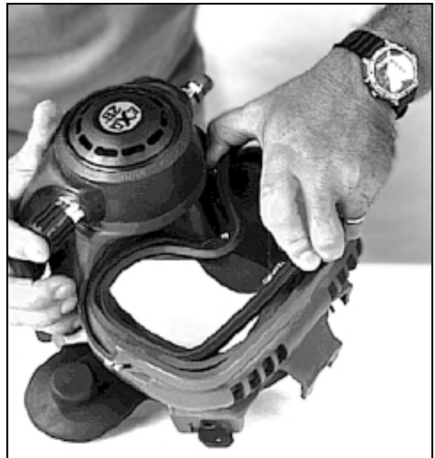
Install the right side of the lens rim into the channel of the rubber on the mask seal.
